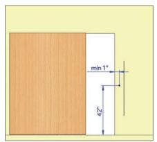
For drywall opening with 1/2" drywall (gypsum board), min. 2" door overlap is needed to install BD4000 privacy lock. The lock bore center must be at least 1" from wall edge; align strike with lock.
