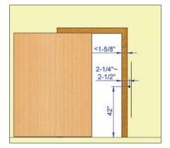
Do not install lock on casing that is less than 1-5/8" wide. Drill lock bore at least 2-1/4" from edge. For this type of installation, door overlap must be at least 3". Align strike with lock.
