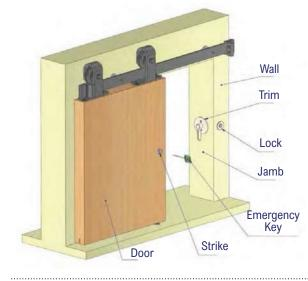
Installation based on barn door application where doors are hung on the  $\ensuremath{\text{OUTSIDE}}$  of the room.
